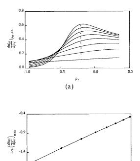
Fig. 20. (a)  $d\bar{n}_{02}/d\bar{\mu}_{\rm V}$  along the line  $\bar{\mu}_{\rm H}=0.5$  for finite sizes with  $\delta=0$ . Developing peaks indicate a transition from  $I_0$  to the quasicrystal phase Q. (b) A log-log plot of peak heights in (a) versus system sizes. The almost linear behavior suggests a continuous transition, consistent with the prediction of Landau theory.
